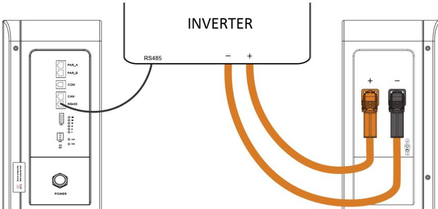
Schematic diagram of connection with inverter - recommended connection
