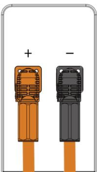
The power cable is connected with the Powerporter through a quick-plug interface, and connected with the inverter through a ring terminal.
